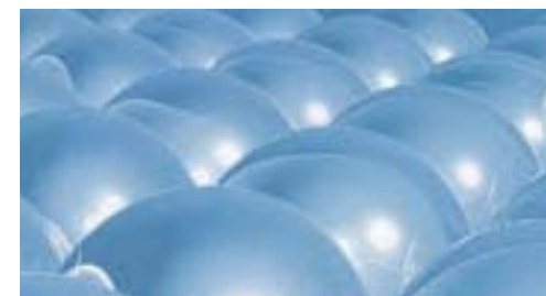
Spacers that maintain uniform thickness of the liquid crystal layer
